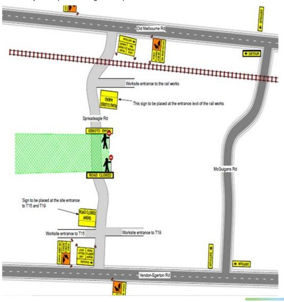
Traffic speeds will be reduced down to 40 kph around the area and Spreadeagle Road will be periodically closed during crane movements. Please take note of speed limits and construction traffic on Spreadeagle Road. Detours will be place along McGuigans Road.
