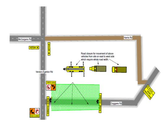
Traffic speeds will be reduced down to 40 kph around the area of the crane movement. Detours will be in place along Harris Road and Yendon Egerton Road.
